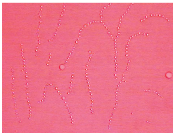
Figure 1. Chains of isotropic droplets on a \sim 100 nm thick smectic membrane prepared using a 4 wt% azoxybenzene-derivative D' 55 mixture and liquid crystal ZLI 5014. Observations were carried out in unpolarised light in the temperature region near the clearing point, T \sim 66^\circ\text{C} . The average size of the droplets varies from 10 to 15 nm (colour version online).
